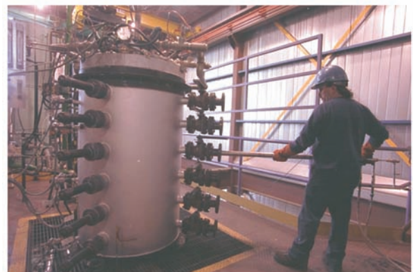
CEPG staff performing temperature measurements on the vertical combustor
