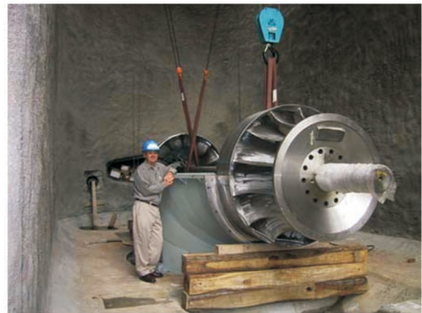
Improved Camelback Francis Turbine in the No. 11 Powerhouse, Energy Ottawa
